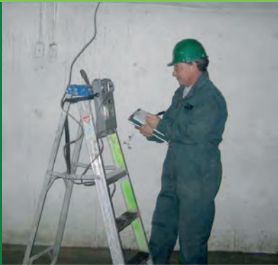
Post-Tech® PT Corrosion Evaluation determines the corrosiveness of the environment inside post-tensioned tendons
